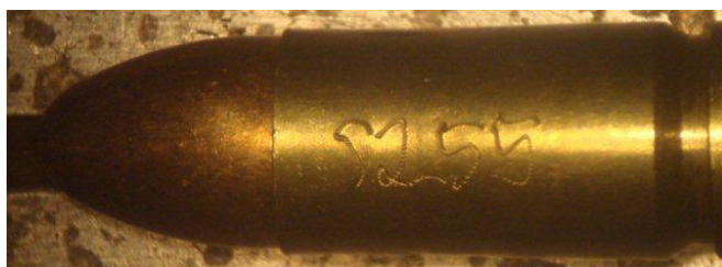
Figure 2a: Unfired cartridge with inscribed identifier
