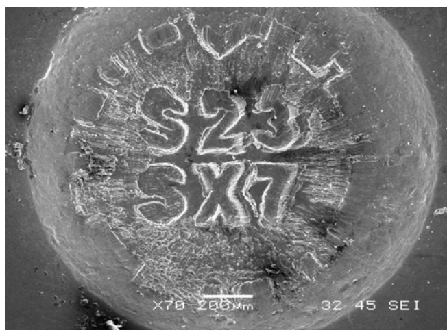
Figure 1: SEM image of a microstamped mark on a cartridge fired by the Sig Sauer. Note the gear code surrounding the alpha-numeric identifier.
